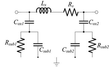
Fig. 3. Lumped element model of a spiral inductor on silicon.
