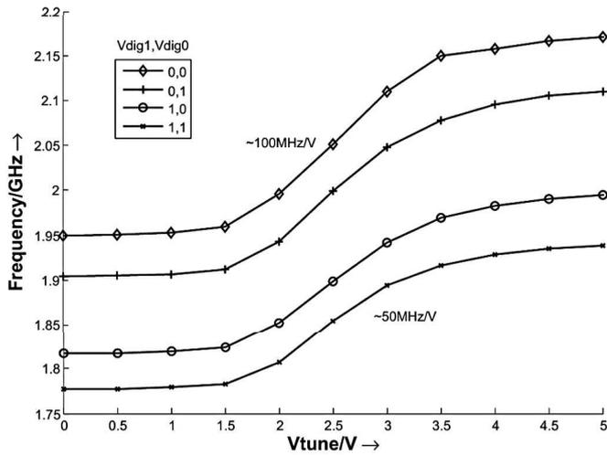
Fig. 7. Measured tuning characteristics of the 2.2 GHz LC VCO.
