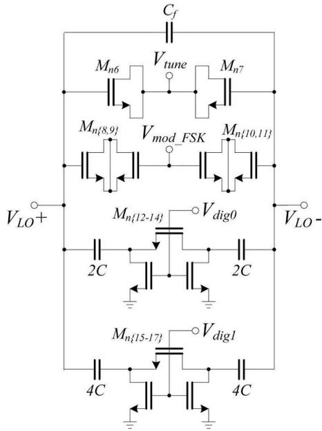
Fig. 5. Details of the capacitor bank in the cross-coupled LC VCO.
