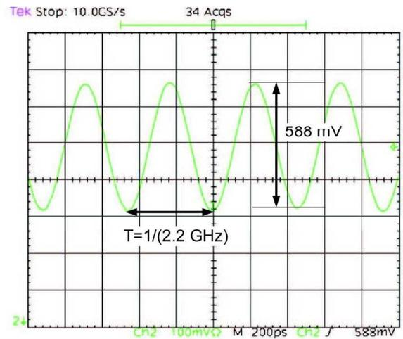
Fig. 9. Real-time scope measurement of the 2.2 GHz cross-coupled VCO at 10 Gs/s.
