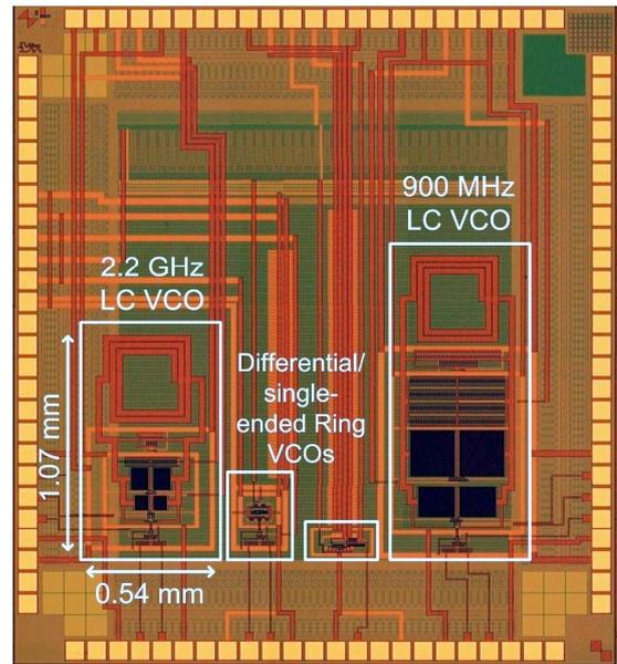
Fig. 1. Die photograph of the fabricated transmitters.
