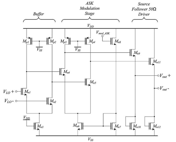
Fig. 6. Output amplifier and ASK modulation stage.
