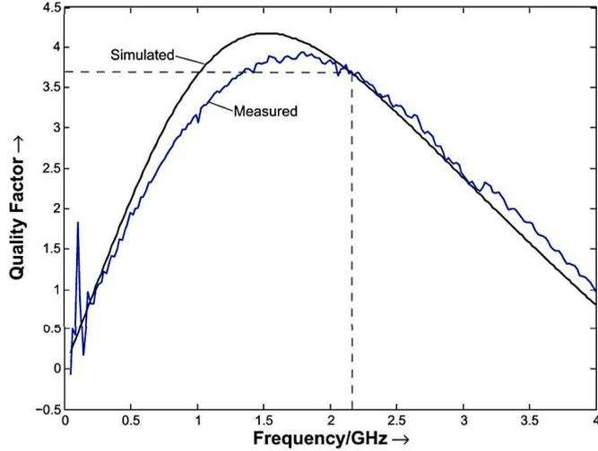
Fig. 2. Measured and simulated inductor quality factor.
