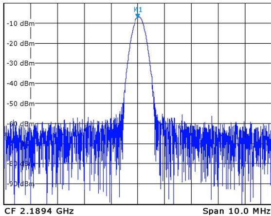
Fig. 8. Frequency spectrum of the 2.2 GHz LC VCO operating at 2.19 GHz. (Frequency response shape is limited by the radio-bandwidth filter of the spectrum analyzer.)
