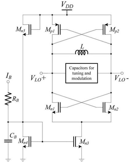
Fig. 4. Schematic of the LC VCO core.
